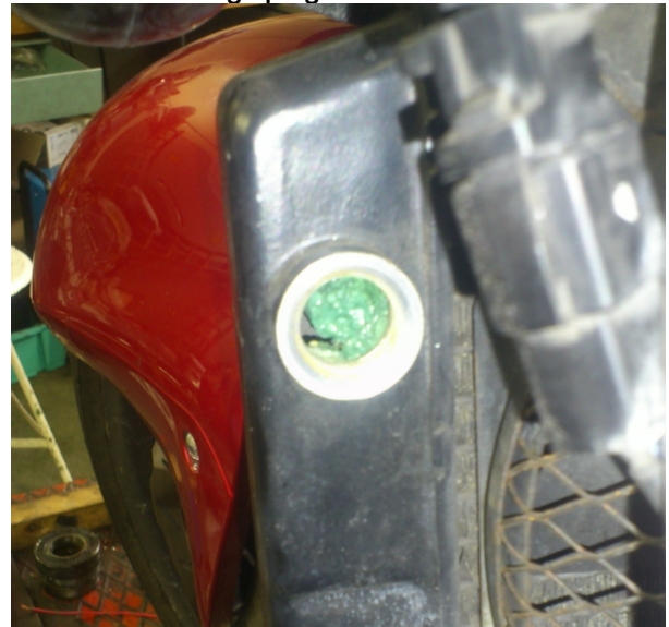
gritty greenish green Sludge plug in the radiator
