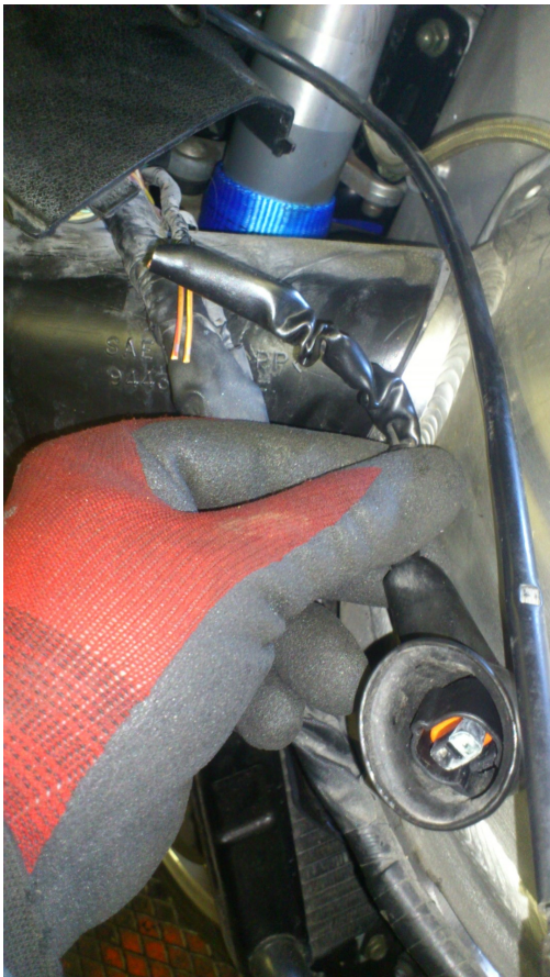
Pic. 3 - plug wire cut off (main harness left side / front, above the air duct)
